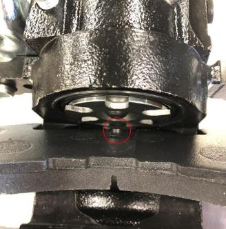
Install the rotor using 2 lug nuts to retain it. **Kits with parking brake calipers** should be checked to confirm the pad is seated flat against the piston face, with the boss of the brake pad lining up with the notch in the piston face.
