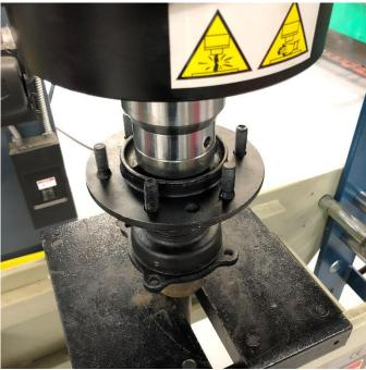
After removing the axle, thread the 4 flange nuts back on flush with the tops of the studs, and remove the studs by driving out with a hammer. This will allow the backing plate to be removed and discarded. Optionally, a new wheel bearing can be installed at this time. The axle can now be reinstalled into the bearing on a press by supporting the bearing as close to the center as possible.
