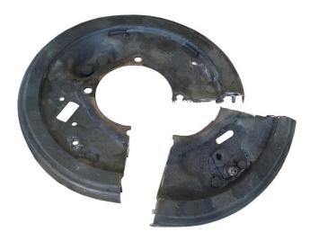
Reinstall the retaining ring, and then install the axle into the housing. **Alternatively to pressing off the bearing:** the user can choose to remove the studs, slip the backing plate down on the axle, then cut a pie shape out as shown using a reciprocating saw or cut-off wheel. When this is done, it is possible to remove the backing plate without removing the bearing from the axle shaft.
