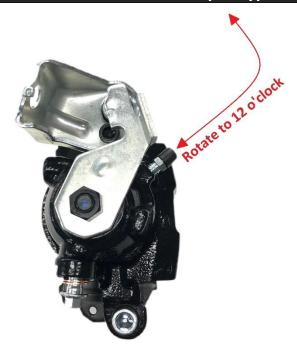
When bleeding this type of parking brake caliper where the bleeder screw is at a 45° angle once installed, we have found that they bleed best when the bleeder screws are at a **vertical 12 o'clock position**. If they are not, then it will be necessary to reposition the vehicle, the axle, or the caliper. **If the bleeder screw is not vertical while bleeding, then you can bleed gallons of fluid through it without eliminating all of the air.**
