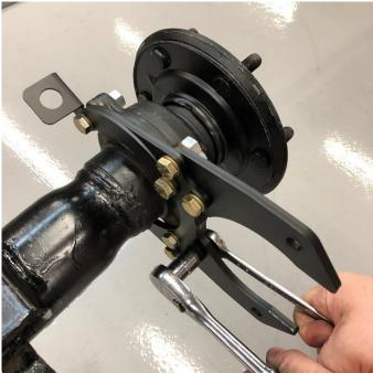
The caliper will be mounted towards the **REAR** of the axle. Install the flange and hose brackets to the inside of the flange using the supplied  $3/8-24 \times 1.5$ " hardware as shown. The caliper bracket will be installed to the outside of the flange bracket using the  $3/8-24 \times 1$ " hardware. Torque to **20 ft-lbs**.
