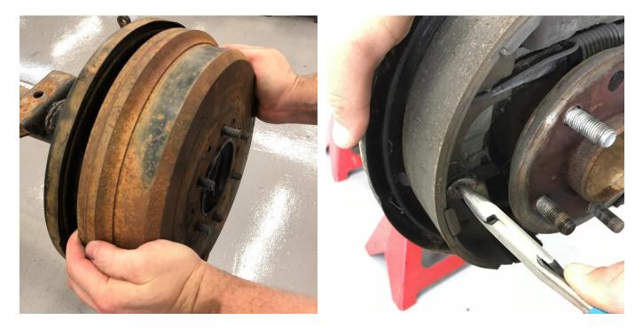
This installation refers to the **passenger side** of the axle. All steps are to be repeated on the driver side. Start by removing the factory drum. It may be necessary use a lubricant around the axle register along with two 5/16-18 bolts threaded into the drum to drive it away from the axle as shown. Once the drum is removed, remove the brake shoe retaining springs (2 places) as shown.
